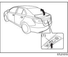
To open the trunk lid, lift it while pressing the trunk lid request switch (1).
